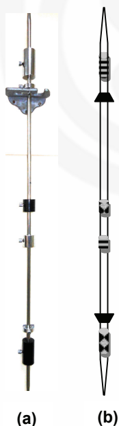
Fig. 7.2: a) Image of Kater's pendulum; b) Schematic diagrams.
