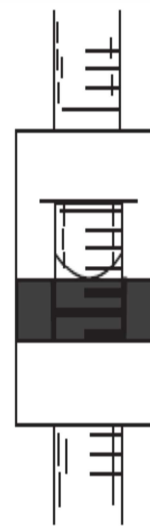
Fig. 1.5: Reading the burette with the use of the parallax card.
