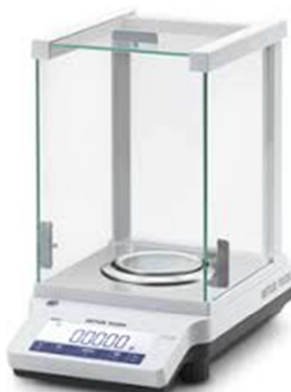
Fig.1.11: Single-pan electronic analytical balance.
